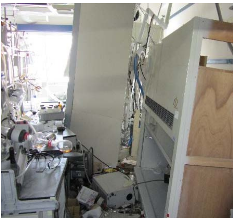
Conditions inside a laboratory: a draft chamber was moved by the earthquake and lab instruments were scattered across the floor.
